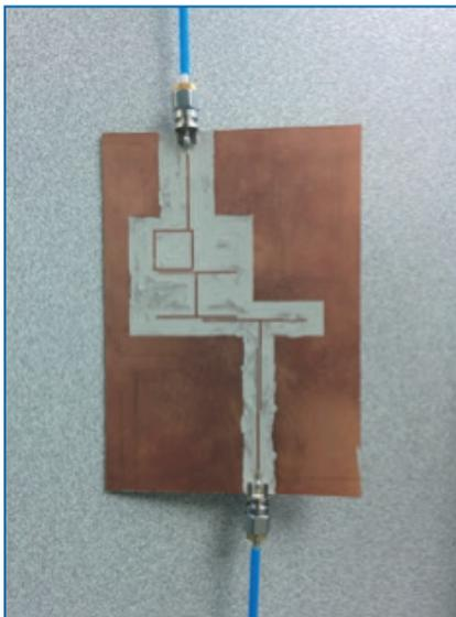
Figure 1: A student's filter design realized with NI AWR software.
