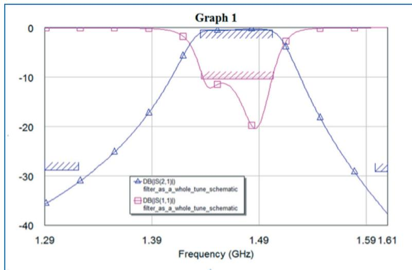
Figure 2: Simulated frequency response of the filter.
