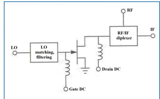
Figure 1: Schematic of the mixer.
