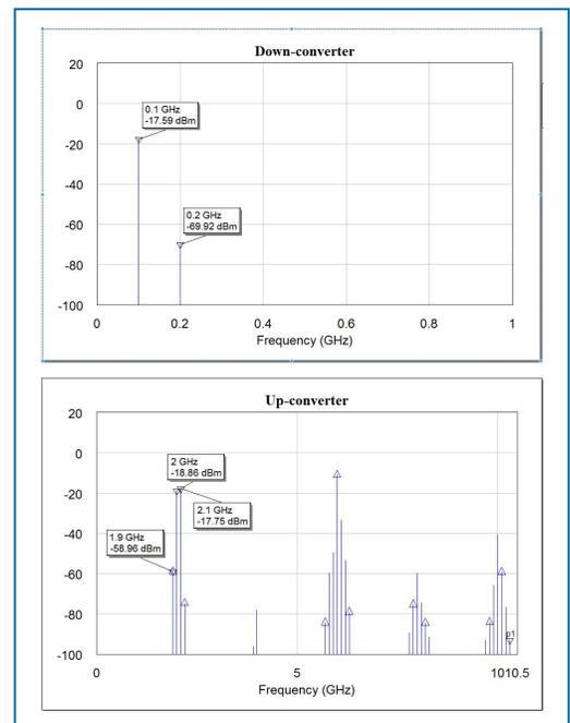
Figure 3. Spectral output of the SSB FET mixer showing mixer products for both up- and down-converted signals.
