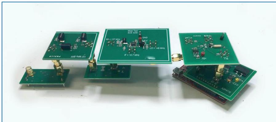
Figure 1: Photograph of student designed receiver being assembled.
